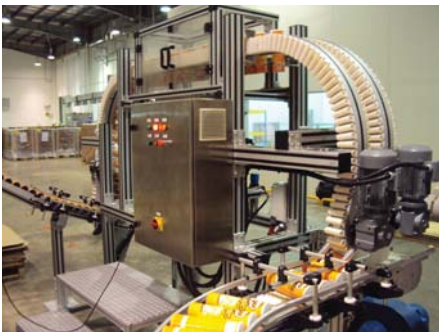
Gripper Conveyor System Intergrated with Can Cleaner to Remove Dust and Particles from Can.
