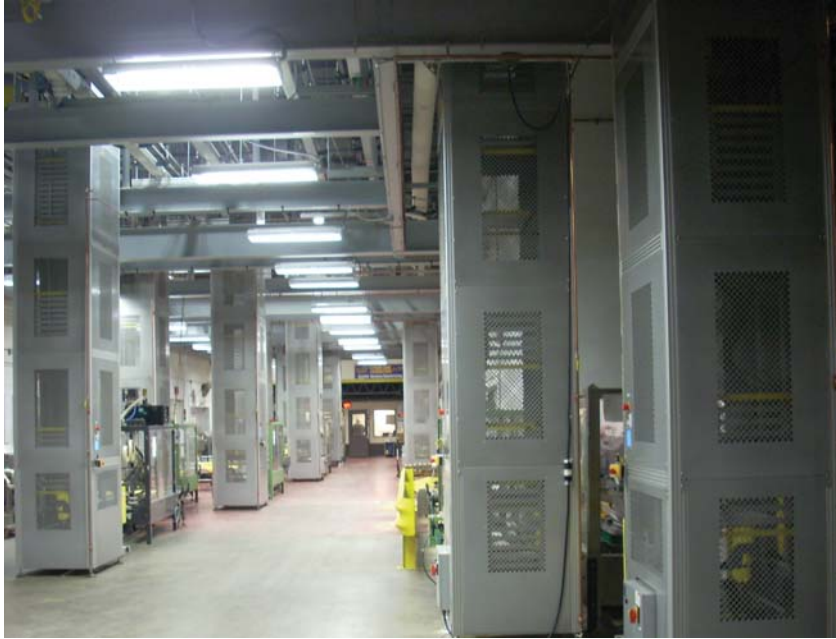
Continuous flow carton / case elevator and lowerator
