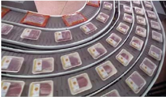
Multi Lane Conveyor System
