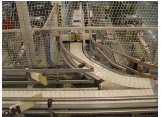
Pneumatic Traffic Controller for Merging
