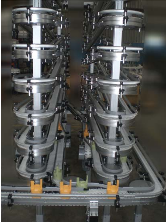
Alpine Conveyor for Puck Storage
