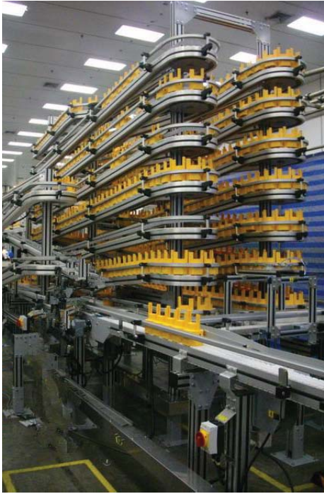
Alpine Conveyor for Puck Storage
