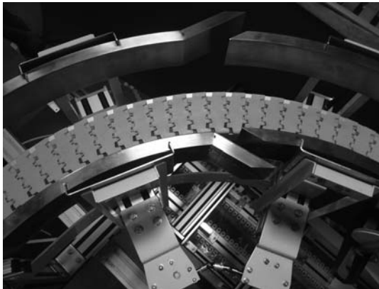
Automated side guide installed at bend section
