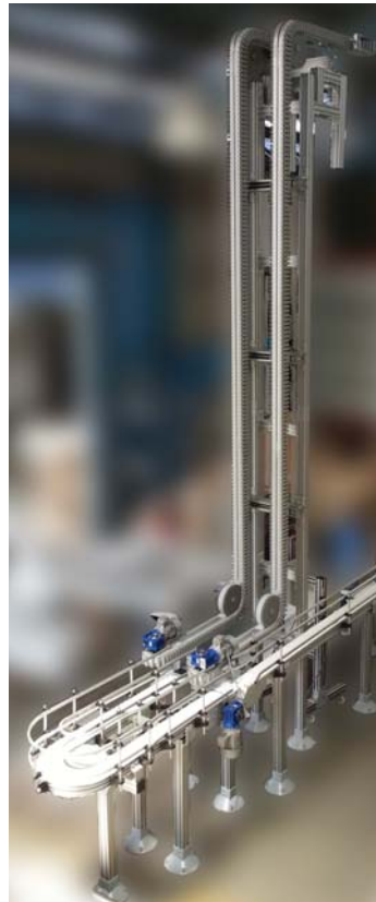
S-Flow Gripper Conveyor to Elevate Carton Boxes
