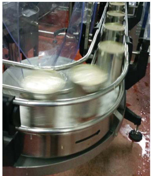
Stainless Steel Conveyor for Wet Environment
