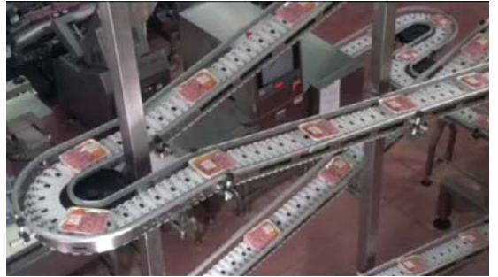
Stainless Steel Friction Incline Conveyor
