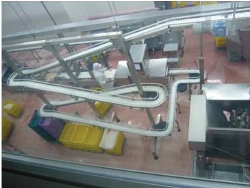
MODU DL Spiral Conveyor for Elevation.
