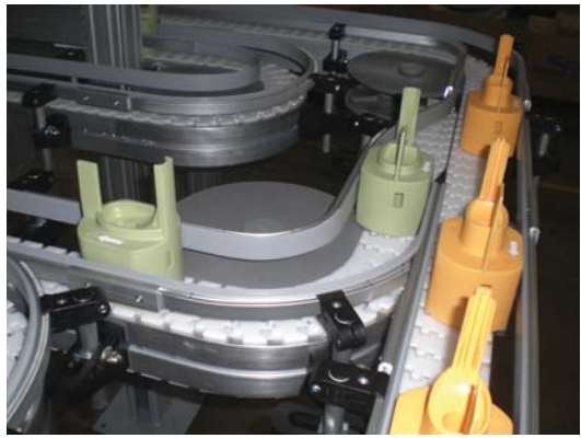
Infeed Conveyor to Alpine Tower.
