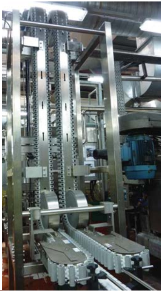
Stainless Steel Gripper for Wet Environment
